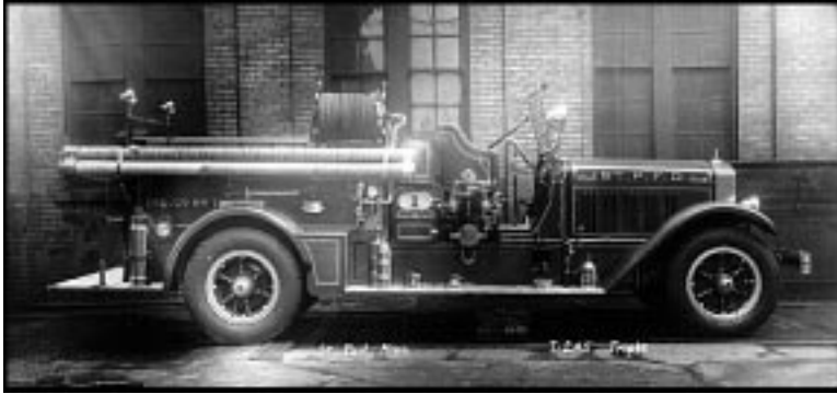
The only pumper purchased in 1931 was this American LaFrance 1000gpm triple combination rig shown in this delivery photo lettered for Engine 7. It was actually placed in service as Engine 4.
